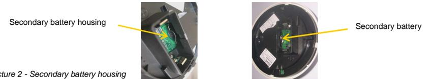
Picture 2 - Secondary battery housing
