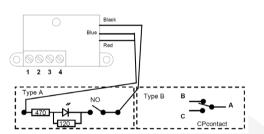
It's possible to connect ONEMICROM10\_AP with call point as Type A connection or Type B connection in base to type of conventional call point used. For Type B connections connect C, NC,&NA of call point with A,B & pin as diagram.
