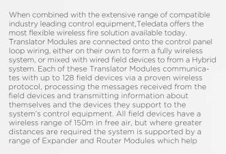
to propagate the radio signals.
